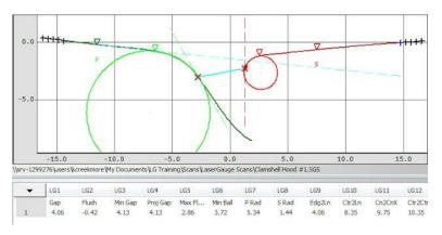
**Instrument** – Hundreds of points are inspected for gap and flush on newly launched models. The instrument must be able to guide the operator to the correct location for each measurement, so the inspection is made in a predetermined order. Each measurement needs to be associated with a unique label or identifier and saved to a data file according to a specified format.
