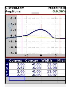
convexity (height), concavity, width, panel mismatch, peaking (panel angle) and weld area.
