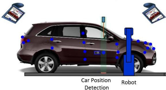
LGAutomation utilizes one robot on each side of the vehicle for left/right side inspection. More robots/sensors can be added as necessary if more measurement points are needed or if the two-robot configuration is unable to keep up with the line speed. Robots can be floor- or gantry-mounted as needed to access the desired measurement locations.
