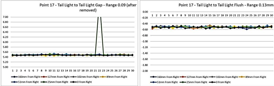
In total, 7 outliers were identified out of the 7560 measurement characteristics acquired during this testing. In each case, the outlier would easily be rejected using scan validation criteria that is set in the sensor firmware. This validation was turned off for this test so that the root cause of the errant points could be ascertained.
