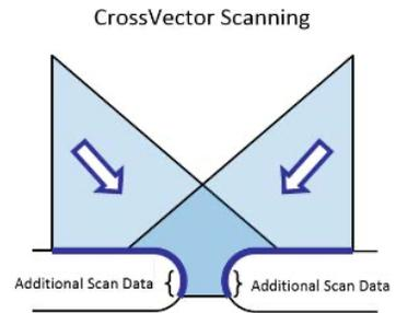
In addition to the Cross-Vector scanning capability, the RS763 utilizes blue-laser scanning technology and advanced signal processing algorithms. This allows the sensor to scan almost all surfaces on an automobile: body panels, headlamps, tail lamps, window glass and chrome. No other gap/flush system has the blue laser Cross-Vector capability.
