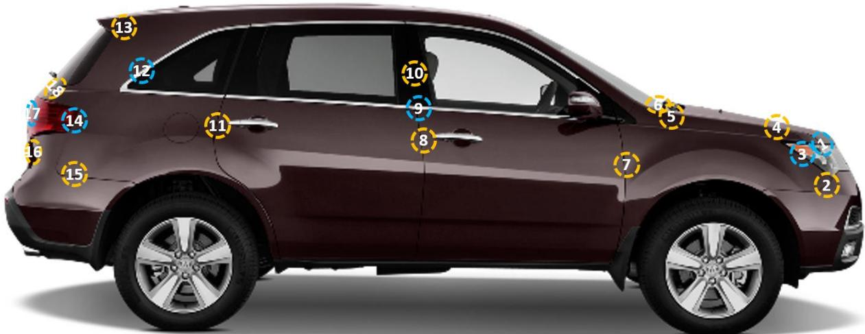
Data was taken at 7 different vehicle positions/angles, with 30 scans per position for a total of 210 scans (18 points/36 characteristics per scan) or 7560 characteristics. Our repeatability goals for these points were as follows:
