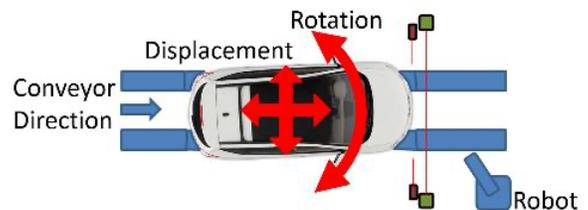
in real-time on a moving line using proven, flexible measurement methodologies. To eliminate any requirement for a stop station or to “pin” the automobile in a known location, a vehicle tracking subsystem tracks the position and orientation of the automobile for real-time robot path correction to ensure that the measurements are taken in the same position each time, regardless of the automobile’s position.
