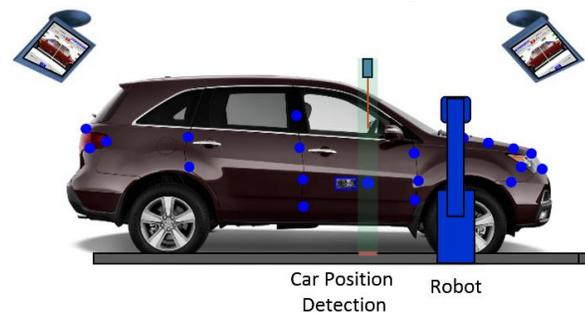
LGAutomation utilizes one robot on each side of the vehicle for left/right side inspection. More robots/sensors can be added as necessary if more measurement points are needed or if the two-robot configuration is unable to keep up with the line speed. Robots can be floor- or gantry-mounted as needed to access the desired measurement locations.
